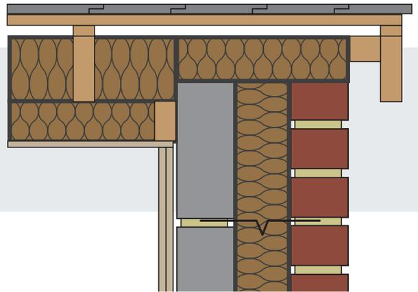
Cavity trays should remain clear of droppings and debris. DriTherm® Cavity Slabs can be easily cut to a chamfer to suit the profile of the cavity tray and ensure no voids are present in the cavity. Slabs can be easily cut with a sharp knife or saw to suit.
