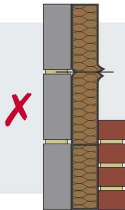
When using small off-cuts, the face of the batts and not the edge, shall be positioned against the wall surface.
