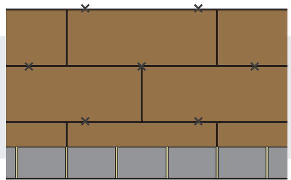
Where cavity insulation batts or slabs start below DPC level, the vertical and horizontal spacing of wall ties should be compatible with the spacing to be used above DPC level.
