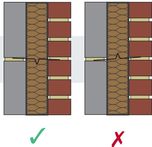
Where extra ties are required, e.g. at the side of openings, DriTherm® Cavity Slabs should be cut and fitted carefully around them. When off-cuts of DriTherm® Cavity Slab are needed, the batts can be cut with a long bladed knife or fine tooth saw.
