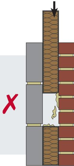
Do not position DriTherm® Cavity Slabs on batts that have not been cleaned of mortar droppings.
