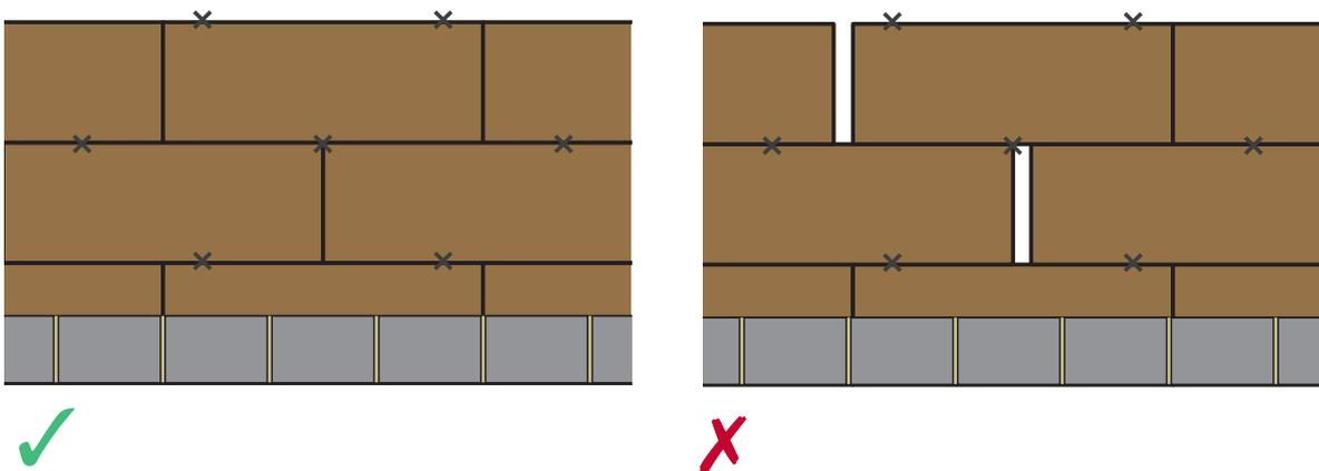
Any cutting and fitting should be neatly done, so not to distort the layers of glass wool which could compromise the material's performance.
