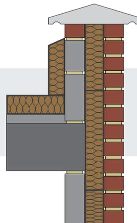
At eaves, cavity insulation should terminate at the top of the wall to meet the insulation at ceiling level. This ensures continuity between the wall and roof insulation and prevents any unwanted heat loss at the junction.
