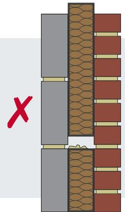
Do not tear or impale DriTherm® Cavity Slabs. If there are protrusions into the cavity, DriTherm® Cavity Slab should be carefully cut to fit, particularly where there are extra wall ties around openings.
