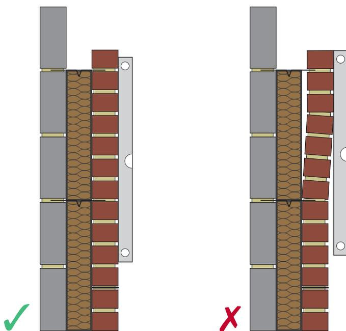
Knauf Insulation and NHBC recommend a cavity of uniform thickness is maintained throughout the construction and therefore we do not recommend rough stone to be used. Where natural stone is specified, we recommend the stone is cut to face to ensure the resultant cavity is uniform and parallel and stone is in accordance with this recommendation or alternatively a backing block is used in the outer leaf.
